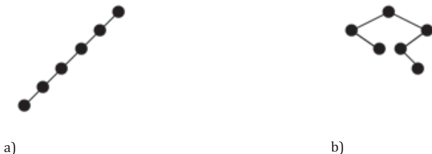
Figure 15. Trees with which, when rolled with the CCW() algorithm, will exhibit a) worst-case time complexity; and b) best-case time complexity
