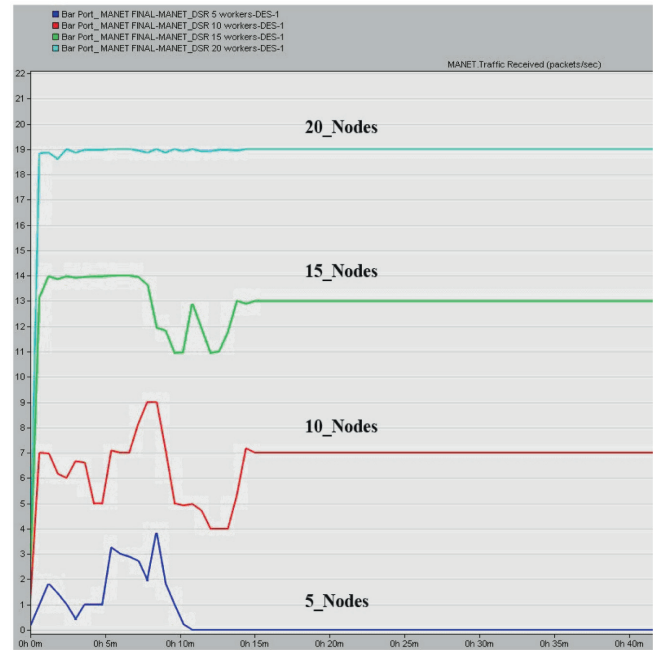
Figure 5. Traffic received by destination in the case of DSR routing protocol in MANET for the scenarios with 5, 10, 15 and 20 nodes (Source: own)
