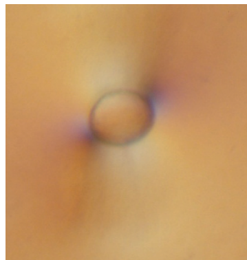
Fig. 5b. The same as in Fig. 5a but polarization contrast is used instead of phase contrast. The water tree is practically invisible.
