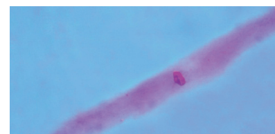
Figure 4d. Bow-tie water tree of 1.5 mm length growing from a small inclusion. In this case the image contrast is provided with the help of the so-called Reihberg illumination (color variant of the dark field microscopic method) – “optical staining” based on the use of light filters instead of staining the insulation slices containing water trees (see photo in Fig. 4a-c and Fig. 6) with a special staining agent.
